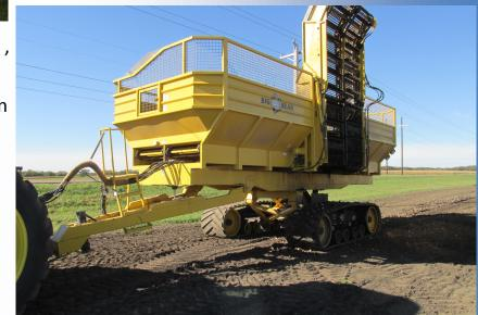
**Proven unloading system:** all sprockets , chains , shafts, hydraulic motors, and unload conveyor are sourced from **ROPA** and performance proven on the **Tiger**.
