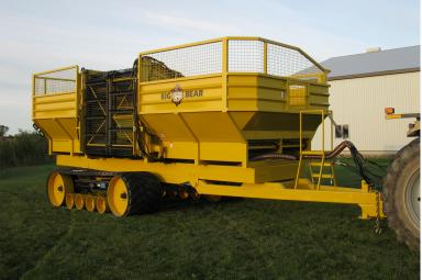
the Maus Drive beside, instead of tracking in front of the pile Good visibility from the cab for unloading Cleaning action by the scrub roller and unload conveyor Center unloading maintains a balanced load
